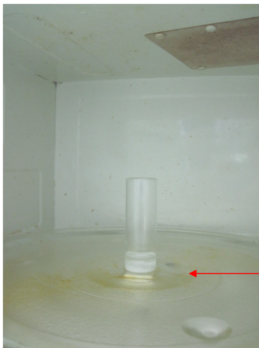
Figure SM X.12. Photograph of the experiment vial in the domestic kitchen-type microwave instrument before the irradiation. The solid in the vial is cyanuric chloride and the liquid N,N -dimethylbenzylamine.
